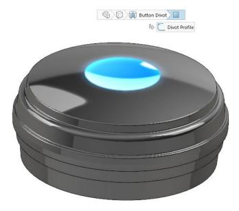
Having selected the face the breadcrumbs dialog can be brought closer to the mouse cursor using the letter D on the keyboard from here the various areas can be accessed. Below the icons are annotated for clarity. Edits are made by right clicking on the item you wish to modify/open.
