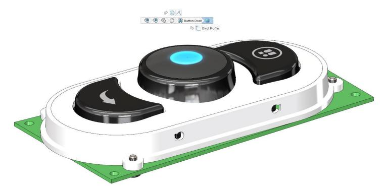
We have access to additional information including mates and the ability to select any sub assembly levels along with the top level assembly, should we wish to open or modify those. Hovering over the mates show a preview of the selected surfaces and can be directly edited from a right click on the area you wish to edit/ open.
